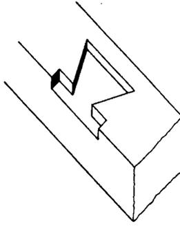
FIG. 37 – Inset dovetail with square entrant shoulders (not to scale).
