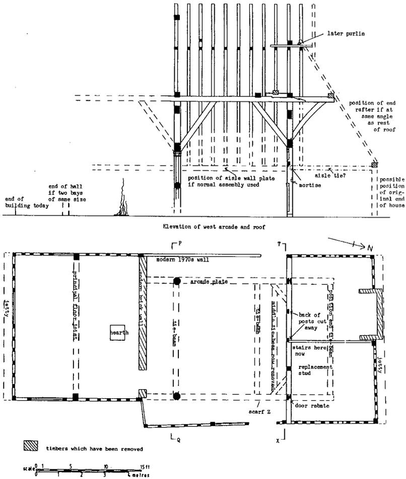
FIG. 30 – Plan of Purton Green as existing now and elevation of remaining part of aisled hall.
