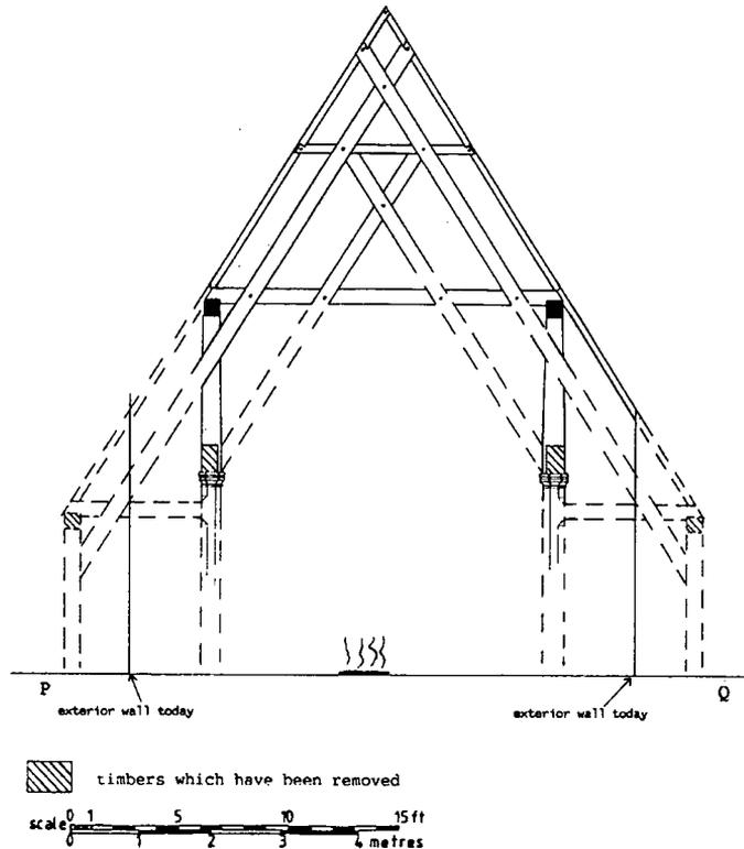
FIG. 31 – Elevation of south side of central truss of aisled hall.
