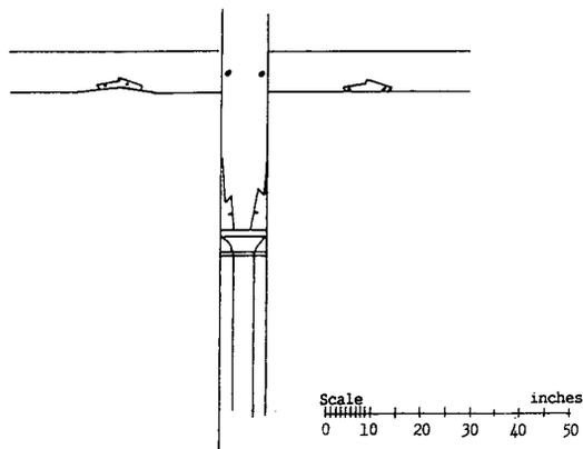
FIG. 33 – Seating for ‘braces’ in post ‘a’ in low end truss (TX).
