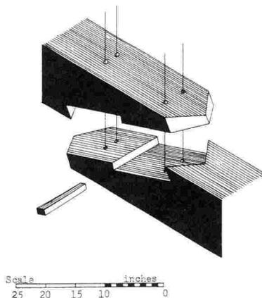
FIG. 34— Stop-splayed and tabled scarf with under-squinted and sallied butts, transverse key and four face pegs in west arcade plate at Purton Green.
