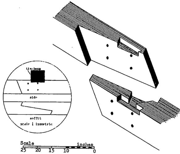
FIG. 35 – Stop face splayed scarf with angled under-squinted abutments and four edge pegs in cast arcade plate under third tie-beam at low end of Purton Green (point Z on plan, Fig. 30).
