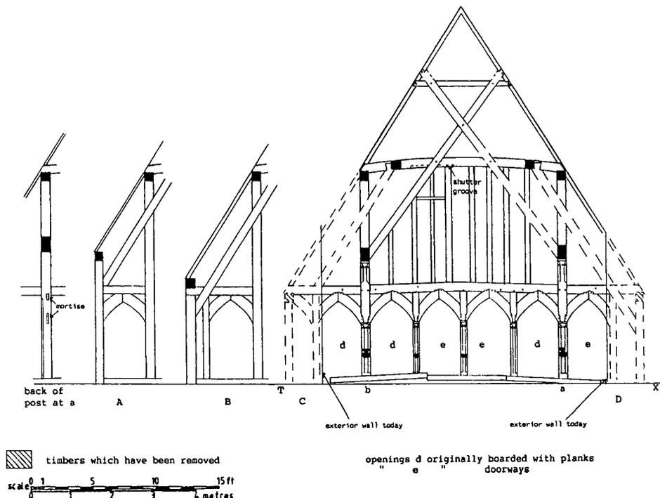
FIG. 32 – Low end partition: (A)–(D) show four possible positions of side walls to original aisled hall.
