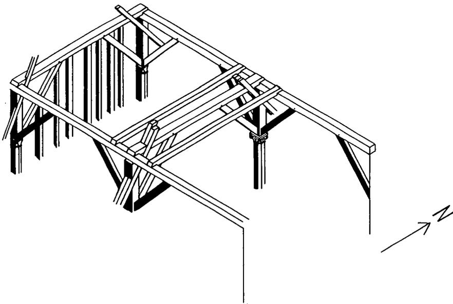
FIG. 36 – Partial reconstruction of aisled hall within Church Cottage and South Cottage, Cookley (south side of central truss based on north side).
