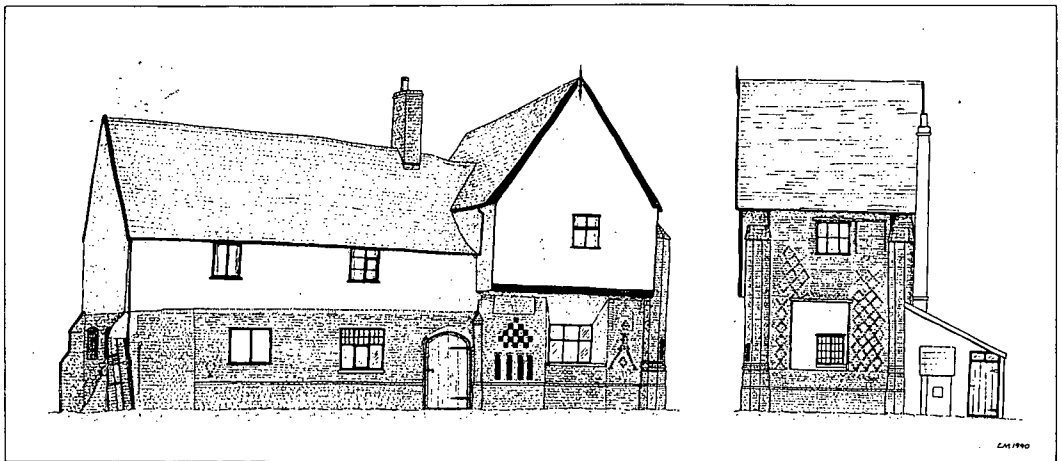
FIG. 33 – Brick House Farm: sketch of the south and east elevations of the house. The building is difficult to photograph and this is an attempt to show the main features of the Early Tudor brick structure. The parlour is in the jettied end to the right.
