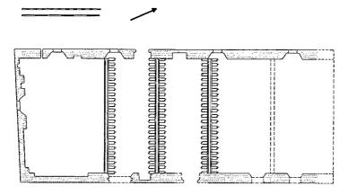
FIG. 21 – Eye, Abbey Farm Barn (EYE 093). Reconstruction of the original ground plan of the Tudor priory bakehouse, showing the unfloored area to the left. Scales in feet (top) and metres.
